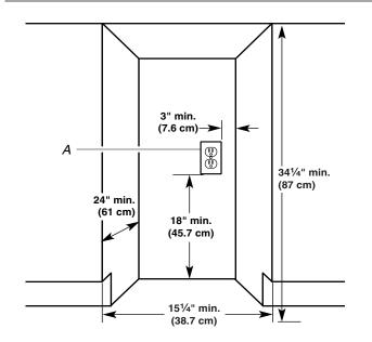
A. Grounded electrical outlet must be a minimum of 3" (7.6 cm) away from surrounding cabinets or nearby walls as shown. It can be placed either to the left or the right side of the product.
